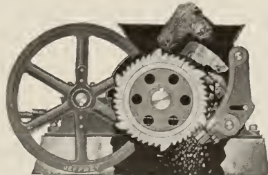
Single Roll Coal Crusher for reducing coal to stoker sizes
